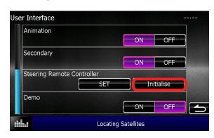
By pushing [Initialise] you can reset the steering remote controller
